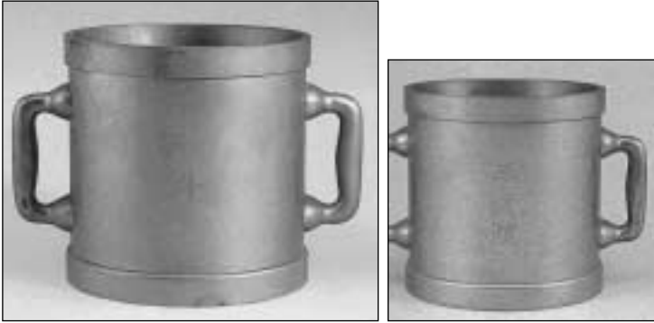
Figure 4 Prototype of Du Produced by Pyeongsikwon (Diameter 21.5cm, height 21.5cm, about 6 l.) “1 du (一斗)” was engraved on the front (left) and “Pyeongsikwon” in the rear.
