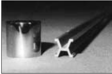
Figure 3 First Standards ( étalons ) of the Meter (right) and the Kilogram (left)
