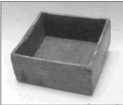
Figure 1 Korean Traditional Dry Measure, mal (Tongyeong, 1895, 26.4x26.4x12.7cm \approx 7,303 cm 3 )
